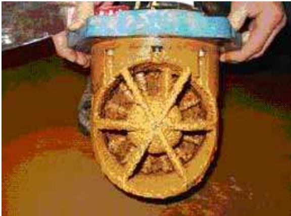
Mechanical water meter after three-month operation
